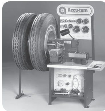
Application for 434466: Mounting of dual wheel and tire assemblies.
